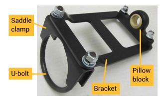
2. With the u-bolt at the bottom with its threads pointing forward and the pillow block hole at the front (12 o'clock) position, slide the bracket assembly down onto the steering column until the u-bolt is over the wider part of the column. Tighten the nuts. Do not overtighten.
