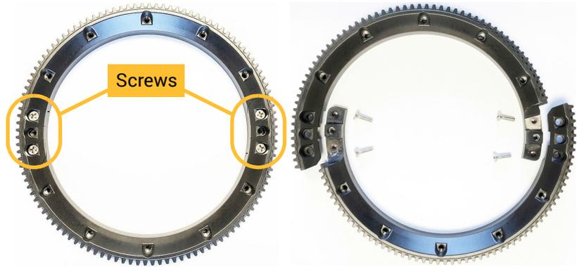
2. With the tops of the gear halves facing upward, place the two halves around the steering column below the wheel. Reconnect the two halves and secure them together with the four screws you removed in the previous step.
