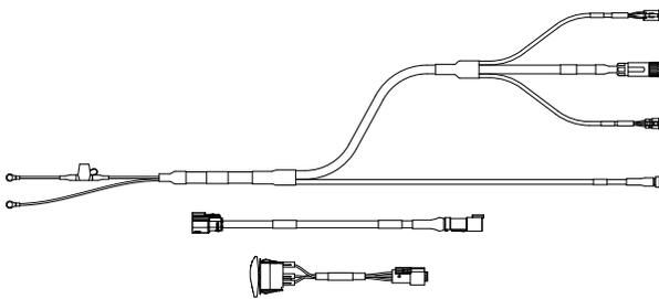
(Top to bottom) Main power cable, RIMU cable,
