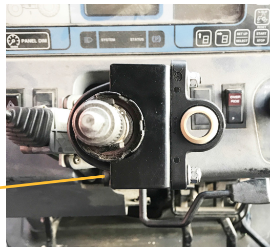
Pillow block at 3 o'clock position
