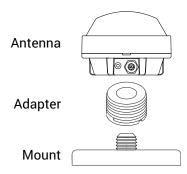
To mount the antenna on the vehicle roof:
