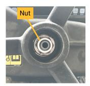
Using a steering wheel puller, rubber mallet, or suitable tool, remove the steering wheel (at right, after). If necessary, consult your equipment dealer if you are unsure of the correct procedure for removing the steering wheel.
